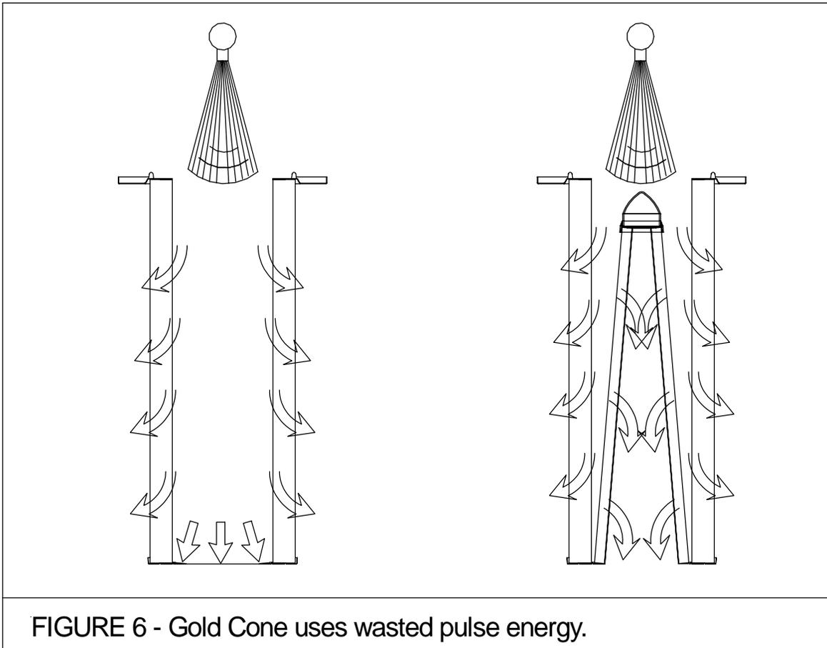
**FIGURE 6 - Gold Cone uses wasted pulse energy.**
