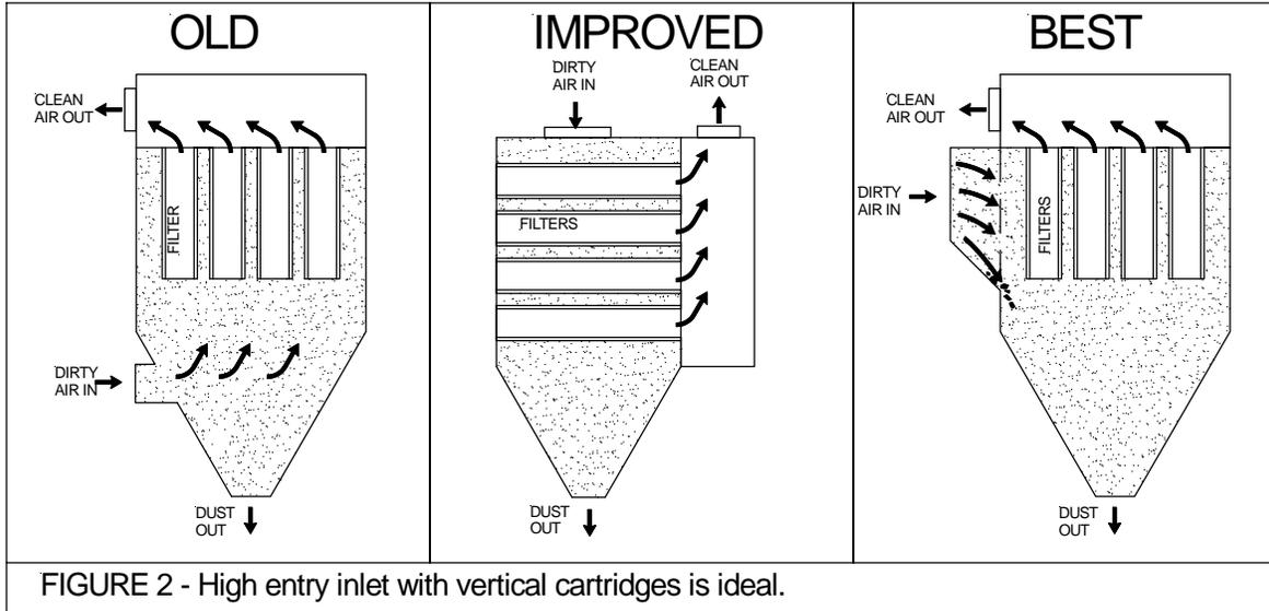
This cross flow effect eliminates upward interstitial can velocities. Since the air is brought into the collector at the cartridge level, there is no longer air flowing upward towards the filters. This system combines the benefit of a down flow style air pattern without turning the filters on their sides and wasting a large portion of the media.
