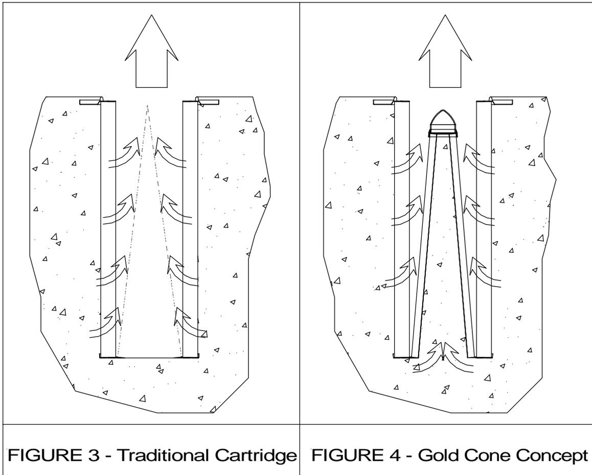
This is a velocity profile of a traditional cartridge on the inside. Notice a natural “cone” forms of dead air. Farr Patent #5,972,059 describes a revolution in dust collection where this dead space is turned into efficient, useful filtration area. Figure 4 shows the same cartridge now with the Gold Cone concept using this dead air space.
