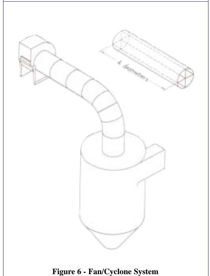
**Figure 6 - Fan/Cyclone System**
