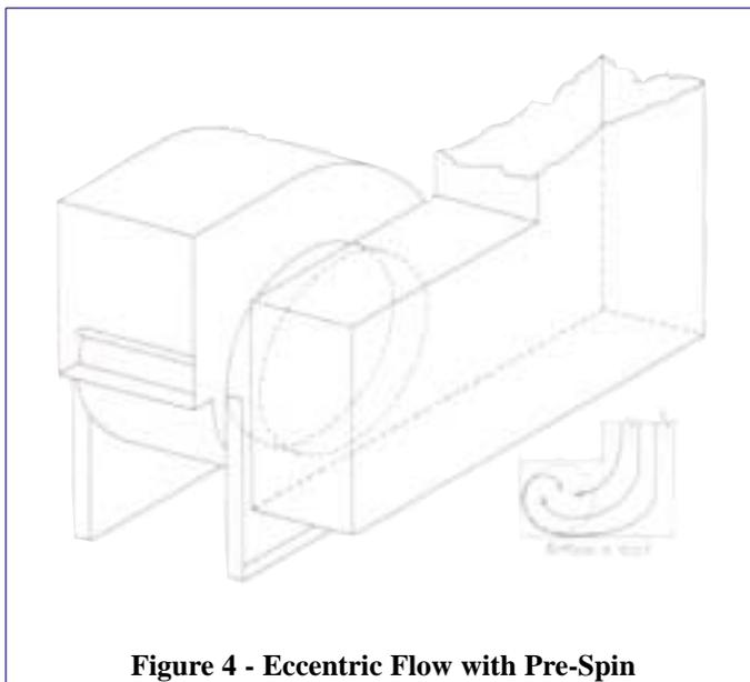
**Figure 4 - Eccentric Flow with Pre-Spin**
