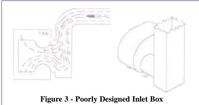
**Figure 3 - Poorly Designed Inlet Box**
