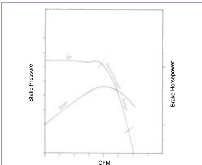
**Figure 7 - Static Pressure Curve for Backwardly-Inclined Fan**
